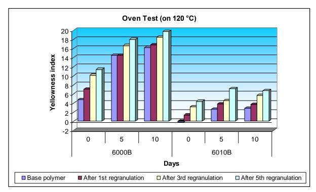
▶ The well stabilized **TIPELIN 6010B** keeps its white colour even after multiple regranulation, which makes the usage of this grade more economic in case of natural products (lower the YI - Yellowness Index, whiter the colour).
